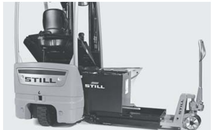
Simple lateral battery replacement with hand pallet truck and battery replacement bed
