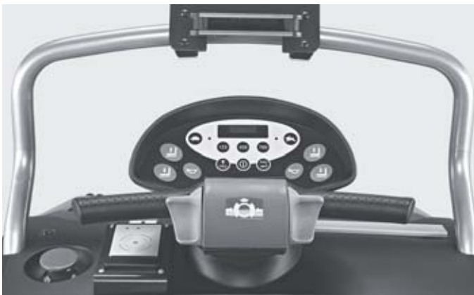
Everything permanently within reach: thanks to the STILL COCKPIT, both left and right-handed users can intuitively operate all of the truck's functions using ergonomic control elements
