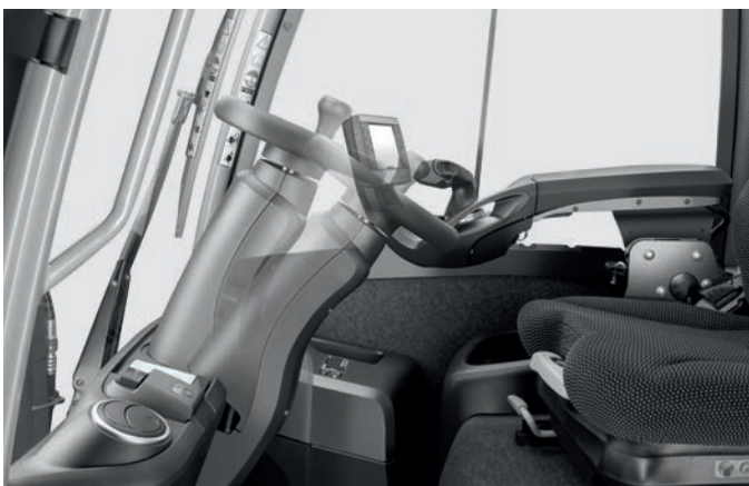
Individual adjustment of the steering column
